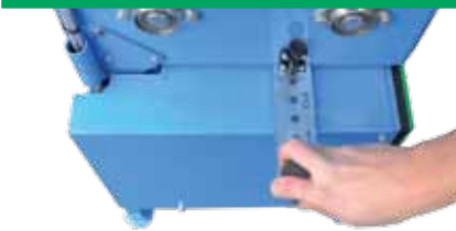
Material- flow regulation via slide-gate
