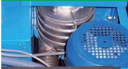
High-power 5.5 kW turbine
