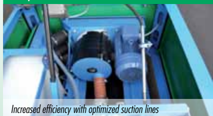
Turbine vibration-damped, low-noise and powerful
