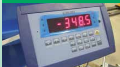
Permanent quality control via weighing unit
