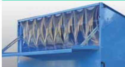
Robust sack tray with dust protection, full width usable
