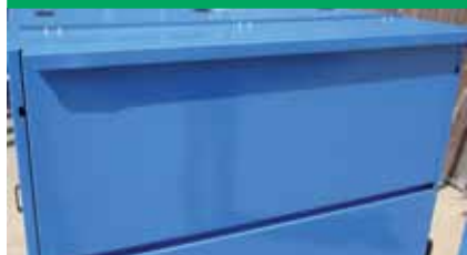
Extension with fold-down lid for dust reduction
