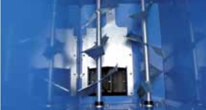
2 hard-wearing shredder shafts ensure optimal loosening
